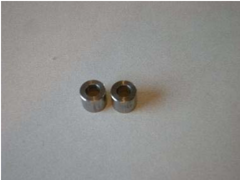
04Y-239 COLLAR, SILENCER MOUNT spacer (Quantity 2) Pictured at the left
