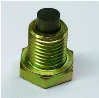
Pictured at the left, 04Y-363 Oil Tank Drain Bolt, 14mm M14 x 1.5mm pitch, 14mm length. Please note; the the depth of boss is about 9mm. If a replacement bolt or plug valve is used, it must be less than 20mm in length.
